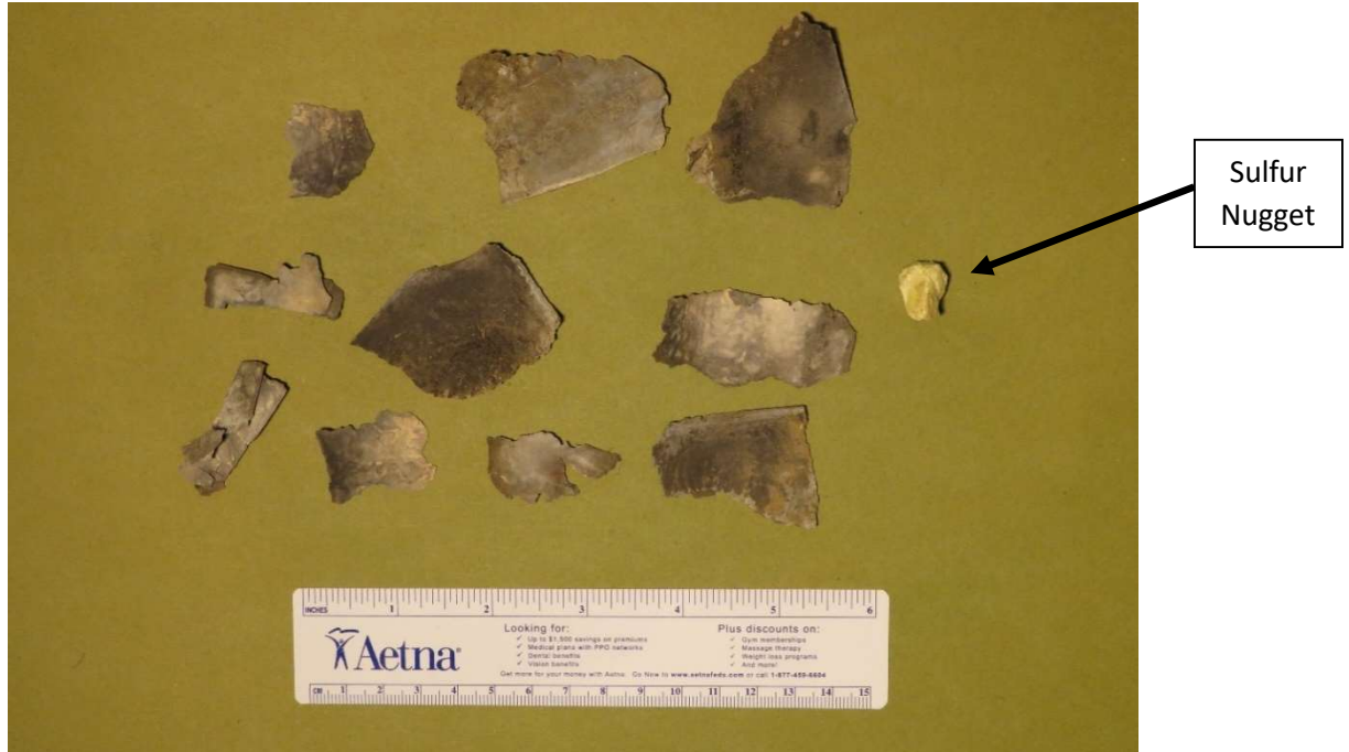
Removed Pieces of Pressed Lead and Sulfur Nugget
